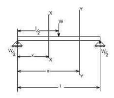
.So the shear force at any X-section would be = W/2 [Which is constant upto x < I/2] If we consider another section Y-Y which is beyond I/2 then
