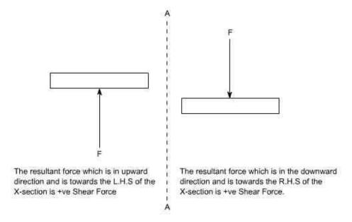
Fig 2: Positive Shear Force
