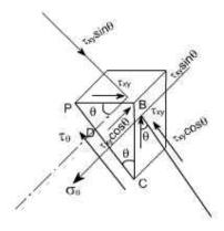
Assuming unit depth and resolving normal to PC or in the direction of  $\sigma_{\theta}$
