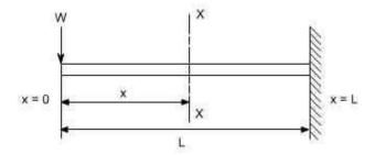
In order to solve this problem, consider any X-section X-X located at a distance x from the left end or the reference, and write down the expressions for the shear force abd the bending moment
