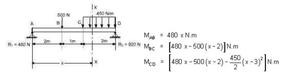
It may be observed that the equation for  $M_{CD}$  will also be valid for both  $M_{AB}$  and  $M_{BC}$  provided that the terms (x - 2) and (x - 3)<sup>2</sup> are neglected for values of x less than 2 m and 3 m, respectively. In other words, the terms (x - 2) and (x - 3)<sup>2</sup> are nonexistent for values of x for which the terms in parentheses are negative.
