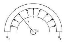
Fig 19.1: Thin ring rotating with constant angular velocity
