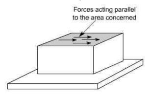
The resulting force intensities are known as shear stresses, the mean shear stress being equal to
