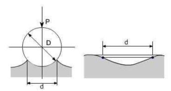
After removing the load an indentation remains on the surface of the test specimen. If area of the spherical surface in the indentation is denoted as F sq. mm. Brinell Hardness number is defined as:
