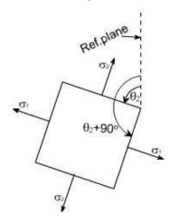
So whenever one of the angles comes negative to get the positive value, first Add  $90^{\circ}$  to the value and again add  $90^{\circ}$  as in this case =  $23^{\circ}74'$
