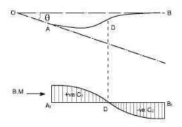
Then, adequate precaution must be exercised in using the above theorem. In such a case B. M diagram gets divide into two portions +ve and -ve portions with centroids  $C_1$  and  $C_2$ . Then to find an angle between the tangentsat the points A and B
