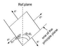
If we just want to measure the angles from the reference plane, than rotate this block through 180° so as to have the following appearance.
