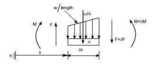
The forces acting on the free body diagram of the detached portion of this loaded beam are the following
