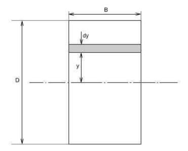
Consider the rectangular beam cross-section as shown above and an element of area **dA**, thickness **dy**, breadth **B** located at a distance **y** from the neutral axis, which by symmetry passes through the centre of section. The second moment of area **l** as defined earlier would be
