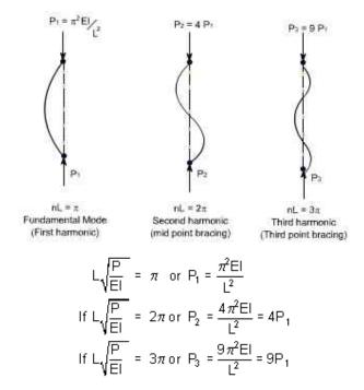
If load is applied sufficiently quickly to the strut, then it is possible to pass through the fundamental mode and to achieve at least one of the other modes which are theoretically possible. In practical loading situations, however, this is rarely achieved since the high stress associated with the first critical condition generally ensures immediate collapse.
