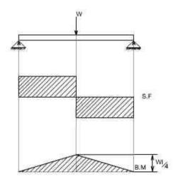
It may be observed that at the point of application of load there is an abrupt change in the shear force, at this point the B.M is maximum.
