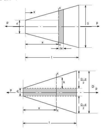
In order to compute the value of diameter of a bar at a chosen location let us determine the value of dimension k, from similar triangles
