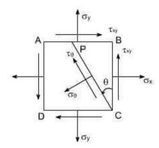
The above system represents a complete stress system for any condition of applied load in two dimensions
