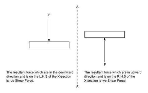
Fig 3: Negative Shear Force
