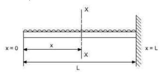
$$\begin{aligned} & \text{S.F}\big|_{x=x} = -w \\ & \text{B.M}\big|_{x=x} = -w.x..\frac{x}{2} = w \left(\frac{x^2}{2}\right) \\ & \frac{M}{EI} = \frac{d^2y}{dx^2} \\ & \frac{d^2y}{dx^2} = -\frac{wx^2}{2EI} \\ & \int \frac{d^2y}{dx^2} = \int -\frac{wx^2}{2EI} dx \\ & \frac{dy}{dx} = -\frac{wx^3}{6EI} + A \\ & \int \frac{dy}{dx} = \int -\frac{wx^3}{6EI} dx + \int A dx \\ & y = -\frac{wx^4}{24EI} + Ax + B \end{aligned}$$
