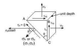
Consider once again the equilibrium of a triangular block of material of unit depth, Assuming AC to be a principal plane on which principal stresses  $_{\rm p}$  acts, and the shear stress is zero.
