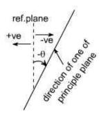
Therefore the direction of other principal planes would be { + 90} since the angle is always less in magnitude then 90 hence the quantity ( + 90) would be positive therefore the Inclination of other plane with reference plane would be positive therefore if just complete the Block. It would appear as
